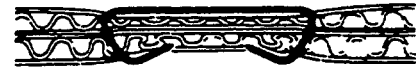
Staple driven completely through two thicknesses of corrugated board and clinched on underside.
